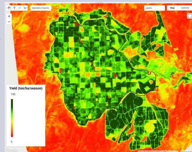
Figure 3 WaPOR derived yield for 2015 for the Wonji irrigation scheme using AGBP and specific conversion factors for sugarcane
